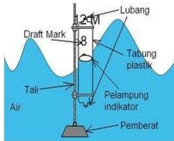
Gambar 2 Alat Reading with floating ball in transparent hose.
